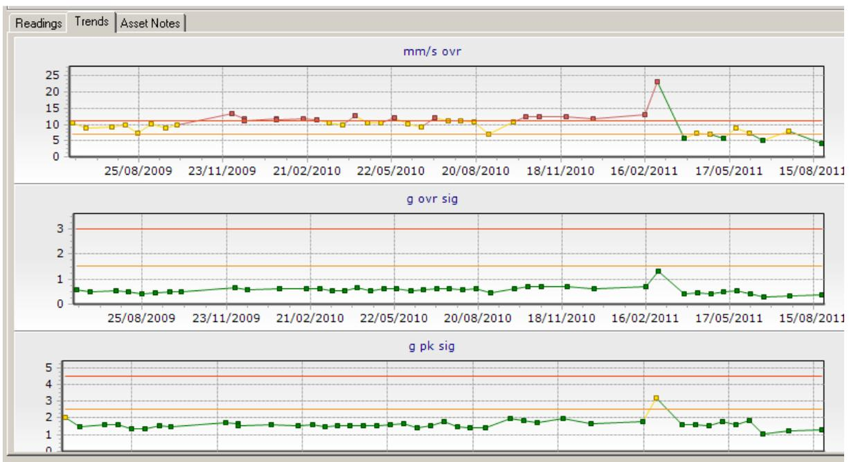
On completion of the FFT analysis, it was found that on both bearings there was a dominant frequency at 99.62Hz with subsequent harmonics, which corresponded to the Pinion/Wheel Gear tooth meshing frequency (Pinion 34T @ 176rpm) and was characteristic of excessive loading or more probably gear tooth wear or misalignment.
