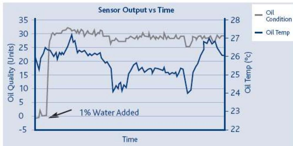
Nevertheless it must be stressed that this oil sensor, like all oil sensors, remains a “blunt” instrument, showing only that “something” is wrong, but not exactly which parameter is in an abnormal state. However, the engineer will have the advantage of a continuous real time early warning system and the added advantage that when the amber sign is alerted an oil change is recommended.
