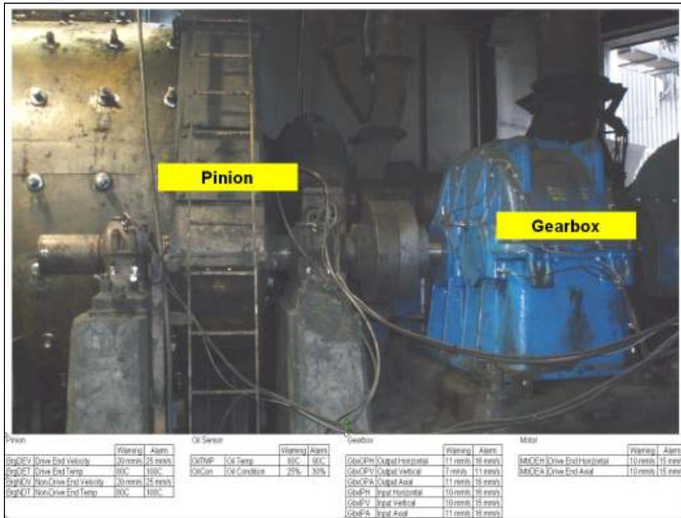
The system detected this increase in vibration (see trends below) and then a detailed FFT vibration analysis inspection was undertaken.
